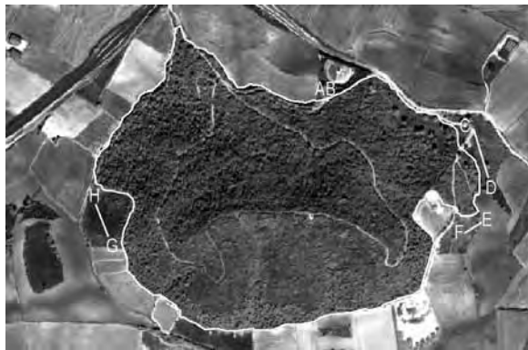
Figure 9. Final delineation of Muskilda forest. Only arc segments AB, CD, EF, and GH have been digitized manually. A color version of this figure is available at the ASPRS website: www.asprs.org .
