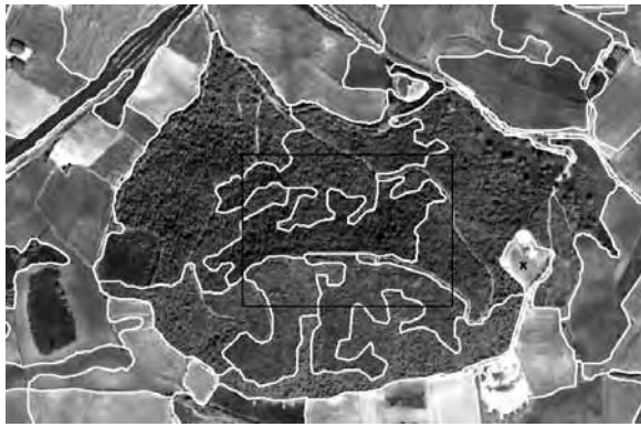
Figure 8. SCRM result used as template for the example in Figure 9 (DMS = 6 ha, MMU = 2 ha, and MVI = 5 m). A color version of this figure is available at the ASPRS website: www.asprs.org .
