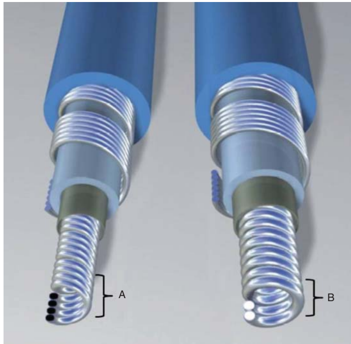
Figure 20.5 Artistic rendering of the construction of a standard bipolar pacing lead (model 5076, Medtronic, Inc.; Minneapolis, MN) (left) and an MRI-compatible bipolar pacing lead (CapSure Fix™ MRI lead, model 5086, Medtronic, Inc.) (right). The standard lead has four tendrils per turn: (A) within the inner coil, compared with two (B) in the MRI-compatible lead. (Source: Reproduced with permission from Medtronic, Inc.)
