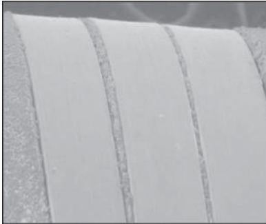
Figure 2.28 Flat shocking electrode construction. (Source: Reproduced with permission of St. Jude Medical, Inc.)
