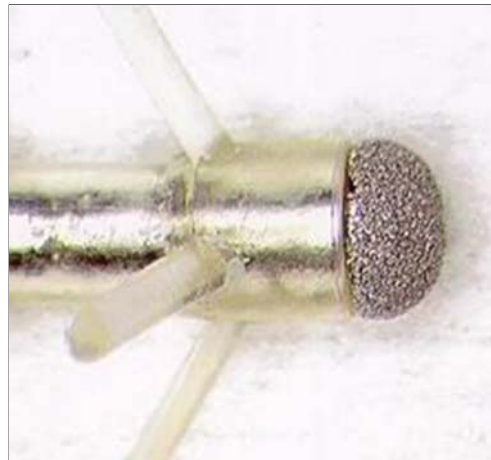
Figure 2.8 Close-up of a porous electrode. (Source: Reproduced with permission of Medtronic, Inc.)
