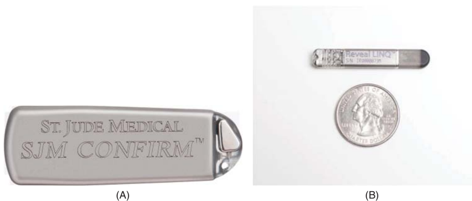
Figure 17.2 (A) Example of an ILR model. (B) Example of a recent small ILR model.
