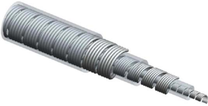
Figure 2.30 Coaxial construction (lead body diameter tends to be high for the multiple layers of insulation, body stiffness is also substantial). (Source: Reproduced with permission of Medtronic, Inc.)
