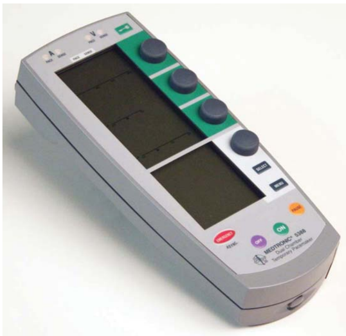
Figure 12.13 Dual chamber temporary pacemaker (Medtronic Model 5388). The dual chamber model can be used where short-term demand (synchronous) or asynchronous pacing is indicated for therapeutic, prophylactic, or diagnostic purposes. The device paces up to 200 ppm, allows ventricular output to 25 mA for high stimulation thresholds and rapid atrial pacing rates up to 800 ppm for managing atrial tachyarrhythmias.
