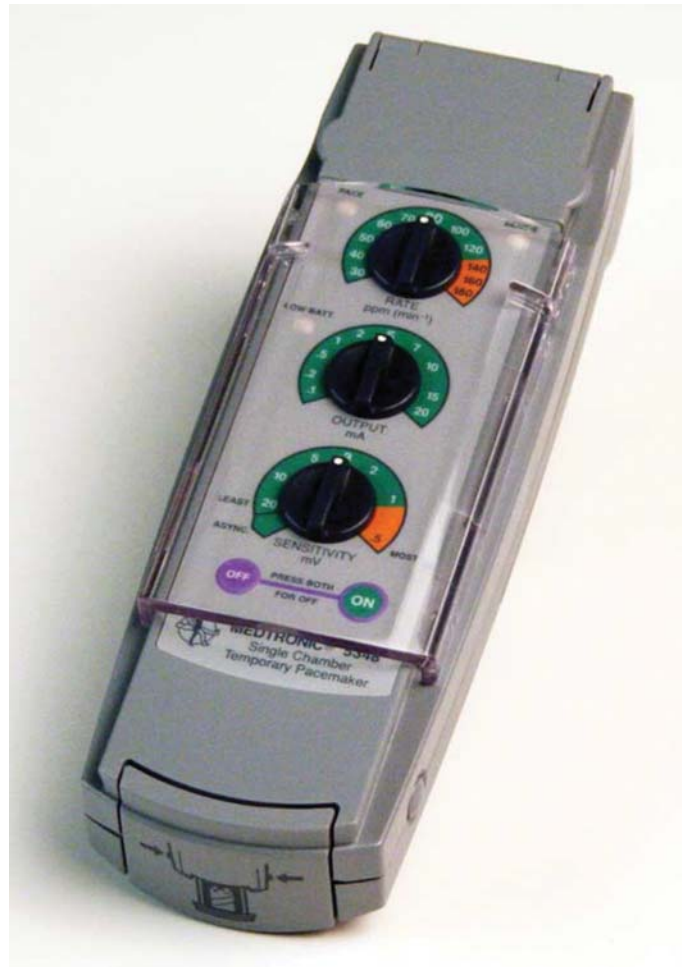
Figure 12.5 Single chamber temporary pacemaker (Medtronic Model 5348) can pace the atrium or the ventricle at rates of up to 180 bpm.
