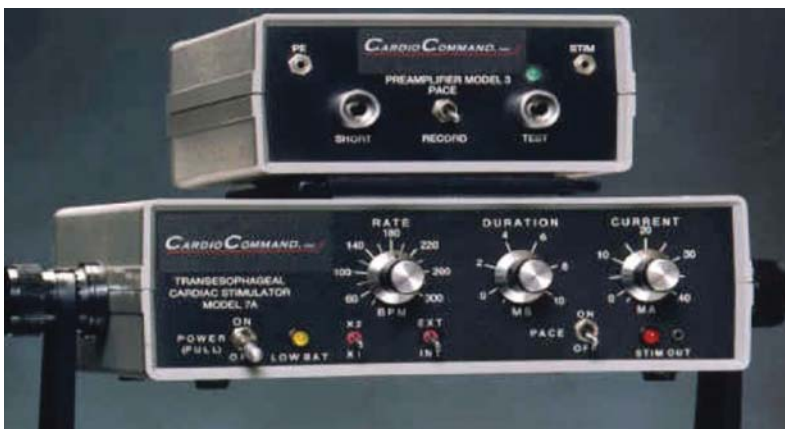
Figure 12.4 Transesophageal cardiac stimulator (Arzco Medical Electronics). The pacing generator transmits pacing pulses from the stimulator to the esophageal catheter. Recording is facilitated with preamplifiers to help eliminate background artifact and allow for simultaneous recordings of esophageal and surface lead electrograms. Asynchronous atrial pacing at rates up to 800 bpm can be delivered.
