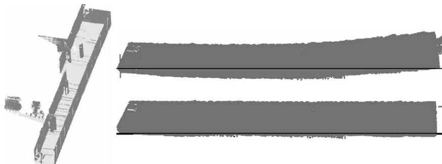
Fig. 17. Left: Map, top view. Right, top: The unconstrained 3D mapping shows a banana-shaped form. Right, bottom: The horizontal justification and the constrained mapping lead to qualitatively correct maps.
