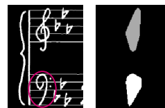
Figure 3. Training on convex hulls circumvents detection problems for symbols consisting of multiple connected components (see f-clef).
