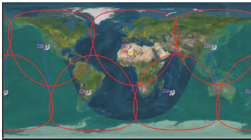
Figure 4.12 Coverage that could be obtained with 6 geosynchronous satellites, each with a 30^\circ inclination, targeting different longitudes.
