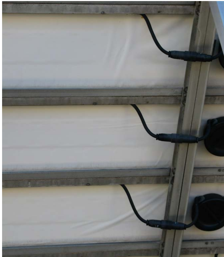
Figure 35: wrinkles caused by the detachment of Tedlar backsheet from the metal foil.
