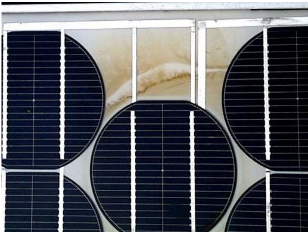
Figure 19: white module with one brown area on internal Tedlar foil.
