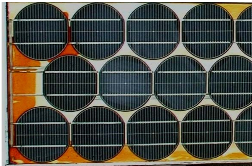
Figure 44: dark yellowing of background in module subjected to DAH.
