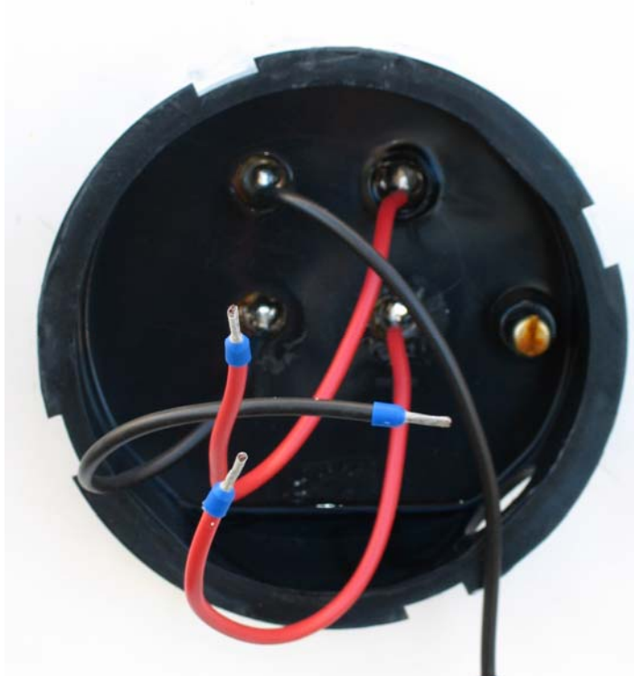
Figure 25: module with detached terminals repaired with soldered cables.
