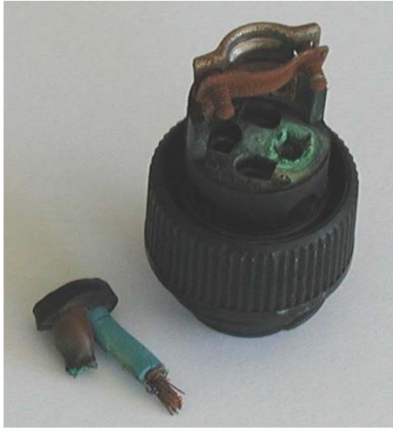
Figure 49: burned cable and damaged connector which caused string fault.
