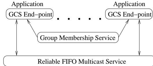
Figure 1.2: The decoupled architecture: GCS end-points provide the Virtual Synchrony semantics by integrating the output of a membership service and a reliable multicast service. Arrows represent interaction between GCS End-points and underlying services.
