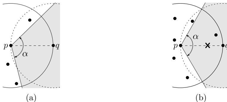
Figure 3-3: (a) \mathbf{p} is \alpha -safe with respect to \mathbf{q} since there is a cone with apex at \mathbf{p} and aperture \alpha containing \mathbf{q} that does not contain a point that is closer to \mathbf{p} than \mathbf{q} . (b) \mathbf{p} is not \alpha -safe with respect to \mathbf{q} since there does not exist a cone with apex at \mathbf{p} of aperture \alpha containing \mathbf{q} that does not contain another point closer to \mathbf{p} .
