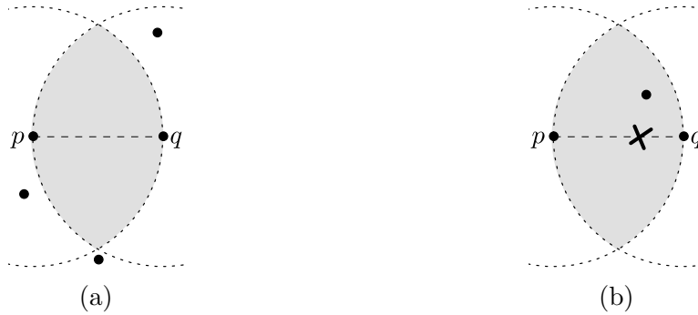
Figure 3-2: (a) \mathbf{p} and \mathbf{q} are RN-neighbors since there is no other point in their RN-region. (b) \mathbf{p} and \mathbf{q} are not RN-neighbors since there is a point in their RN-region.
