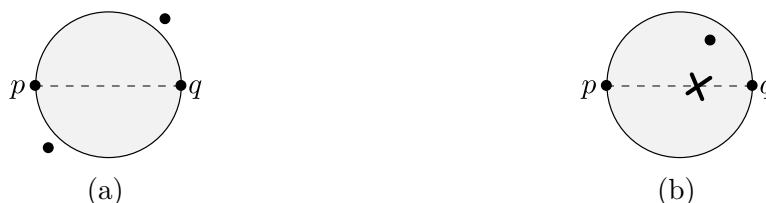
Figure 3-1: (a) \mathbf{p} and \mathbf{q} are GG-neighbors since there is no other point in their GG-region. (b) \mathbf{p} and \mathbf{q} are not GG-neighbors since there is a point in their GG-region.
