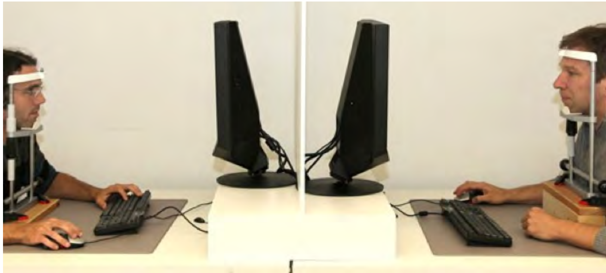
Figure 1. A typical dual eye-tracking experimental setup. Two eye-trackers synchronously record collaborators while they solve a problem.
