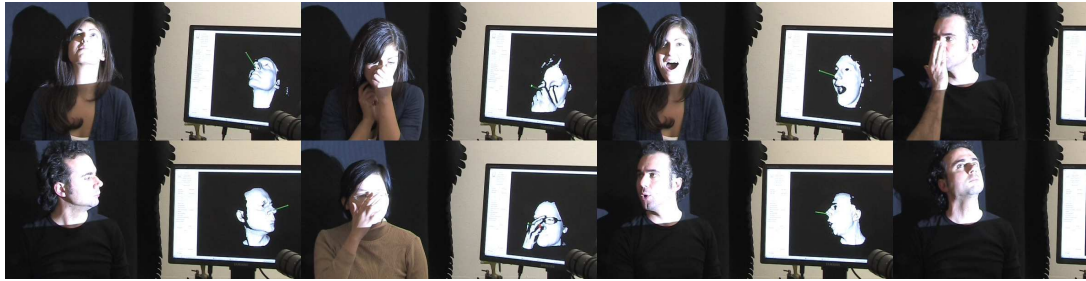
Fig. 14 Example frames from our real time head pose estimation system, showing how the regression works even in the presence of partial occlusions, notably of the nose. Facial expressions also can be handled to a certain degree, even though we trained only on neutral faces.
