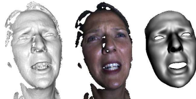
Fig. 24 Example frame from the B3D(AC)^2 database. High quality range scans come together with RGB texture (not used in this paper) and a high definition generic template deformed to match the facial expression in each frame.
