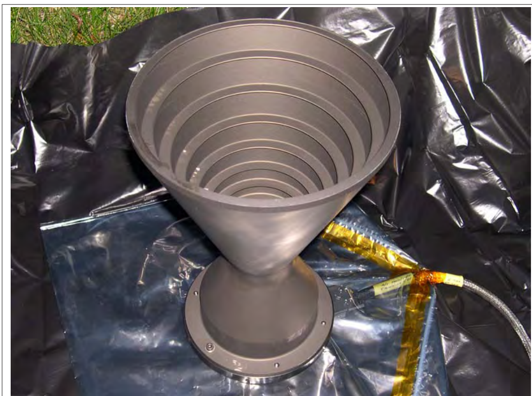
Figure 4.3–2 The light baffle for the CryoSat Star Tracker. This photograph was taken during a night sky test with one of the CryoSat TSar Trackers, which was protected in a clean environment. The baffle itself was manufactured as a flight unit was slightly damaged during handling and thereafter only used for testing.
