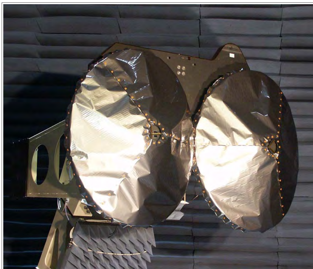
Figure 4.1–1 The SIRAL antenna in the anechoic test chamber during RF testing. The thermal protection, a single layer of germanium-coated mylar, covering the antenna apertures is in place but the Star Trackers have not been fitted at this time.
