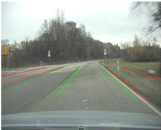
Fig. 13. The outermost left lane is temporarily lost due to lack of road markings.
