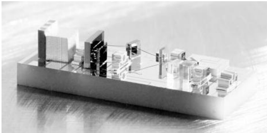
Figure 31. Micro-optical bench (14 mm long) incorporating free space micro optics, a tunable Fabry-Perot filter and fibre optic coupling. Taken from [156].
