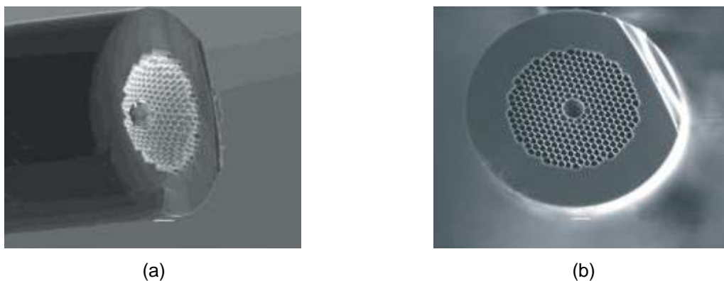
Figure 11. SEM images of a joint between PBGF and standard singlemode fibre that was spliced and then recleaved for examination: (a) at the joint, showing a concave cavity formed by surface tension during splicing, (b) a few mm back from the joint, showing that the integrity of the structure was maintained at that point. Taken from [71].
