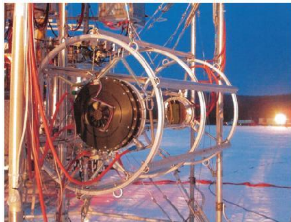
Figure 5. Herriott cell included in a weather balloon payload, used at an altitude of 32 ,000 m to measure methane and water vapour with pathlengths of 74 m and 36 m respectively. Taken from [29].
