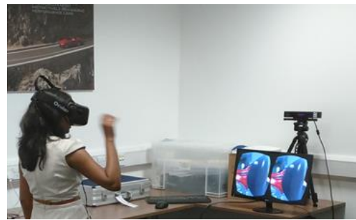
(b) The remote virtual site with a user using an Oculus rift for visualization and Kinect for tracking
