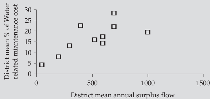
Figure 3.3 District Mean Annual Surplus Flow Versus District Mean Percent of Water-Related Maintenance Cost
