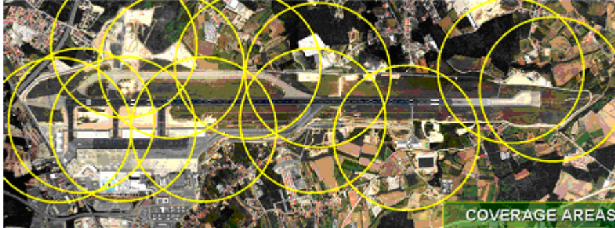
Fig. 6. Distribution of APs and Wi-Fi (802.11a) coverage at the Porto Airport.
