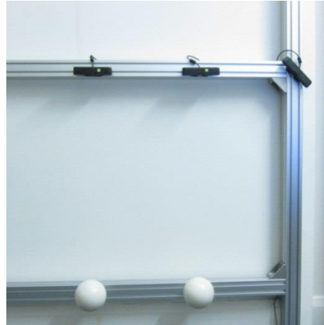
Fig. 4: Experiment set up for testing repeatability. The sensor under investigation is the leftmost sensor. Additional sensors are used to create pattern interference. Two spheres are used as targets.
