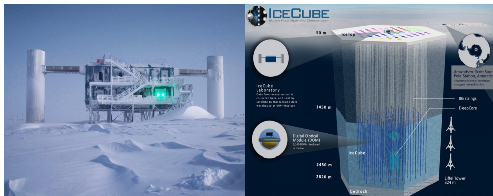
FIGURE 1.3: Left: Picture of the IceCube laboratory (E. Jacobi/NSF). Right: Full schematic of the IceCube Experiment, showing the laboratory at the top and the strings of photodetectors buried 1.5 km away from the top and covering 1 cubic kilometer of ice. (Figure from IceCube MasterClass)
