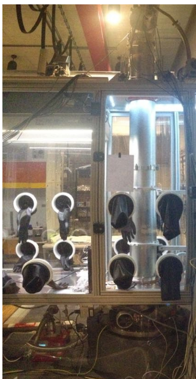
FIGURE 5.1: TUM LAr test stand: In the figure, the lock part inside the glove box and the upper part of the cryostat below the glove box are shown.
