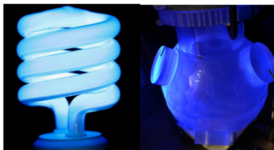
FIGURE 1.4: Left: Compact fluorescent lamp. Figure from [7]. Right: Small scale DEAP-test vessel coated with the wavelength shifter tetraphenyl butadiene (TPB) is lit with a 265 nm ultraviolet (non-visible) LED. Figure from [8].
