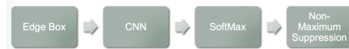
Figure 1: The overview of our object detection system. 1). Edge box algorithm generates proposals. 2). A fine-tuned CNN with object classes plus one background class to extract the CNN features for each proposal. 3) Employ the softmax to give the confidence (score) of all the classes for each proposal (which is typically the last layer of CNN). 4). For each class, independently use the non-maximum suppression (NMS) to greedily merge the overlapped proposals.
