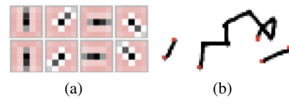
Figure 2: (a) Kernels for detecting line ends. (b) Ends detected on a drawing (highlighted in red).
