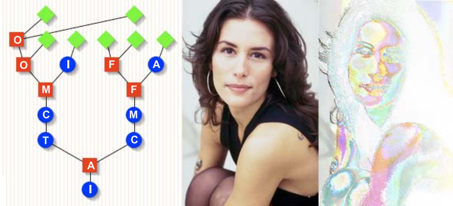
Fig. 1. Example image filter tree consisting of transforms in blue circles: A=Add Colour, C=Convolution, I=Inverse, M=Median and T=Threshold; and compositors in red squares: A=And, F=Fade, M=Min and O=Or. Image inputs are in green diamonds. An example original image and the filtered version are shown.
