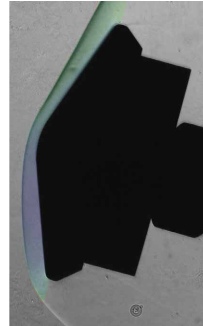
Schlieren image of high-enthalpy CO 2 flow over Mars Science Laboratory geometry.
