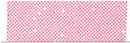
Figure 3: Part of a typical Heliotest strip. The dimensions of a whole test strip are 110mm by 85mm.
