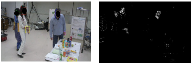
Figure 3: LEFT: frame with bounding rectangles of recognized skin patches and RIGHT: related probability map.
