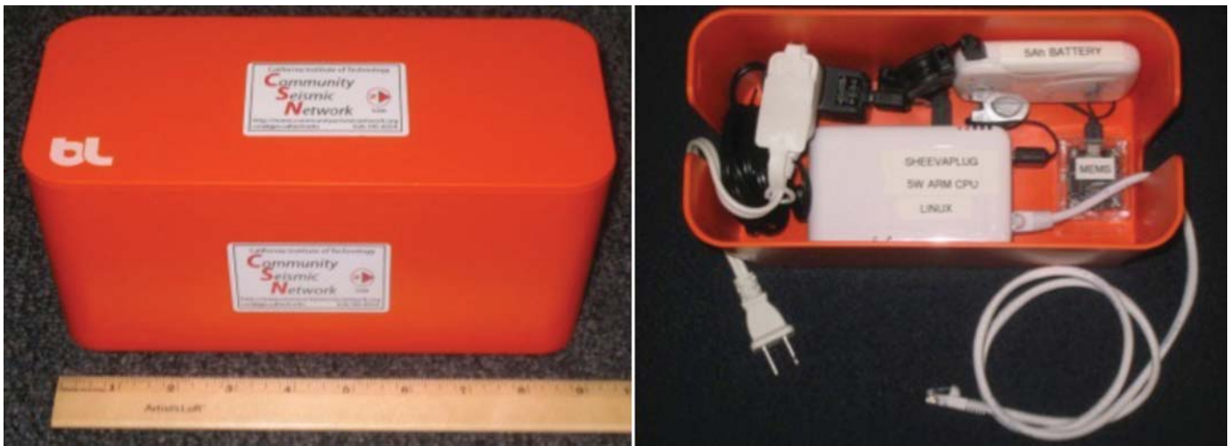
▲ Figure 4. Sensor package: The box contains a Phidget Class-C microelectromechanical accelerometer, and a single-board ARM computer with 512 Mbytes of memory, and a battery backup. The package connects to the Internet by wire and is powered by line power.
