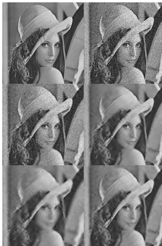
Fig. 2 Comparison of denoising effects of (2.7) with and without a smoothing step. First row (left to right) : clean image, image with 20% Gaussian noise. Second row (left to right) : noisy image smoothed first with a very small c and small time step for 10 iterations, this smoothed image denoised with a larger time step and larger c for 400 iterations. Third row (left to right) : image denoised with the smaller c and larger time step for 200 iterations, image denoised with the smaller c and smaller time step for 1000 iterations
