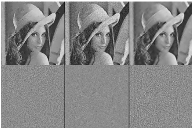
Fig. 4 The Lena image with 20% Gaussian noise added is denoised three ways. First row (left to right): “2nd Order”, denoised with (1.1); “4th Order (1)”, denoised with (2.7) for a short time; and “4th Order (2)”, denoised with (2.7) for a long time. Second row: the method noise for each image. The initial clean and noisy images are the same as in Fig. 2
