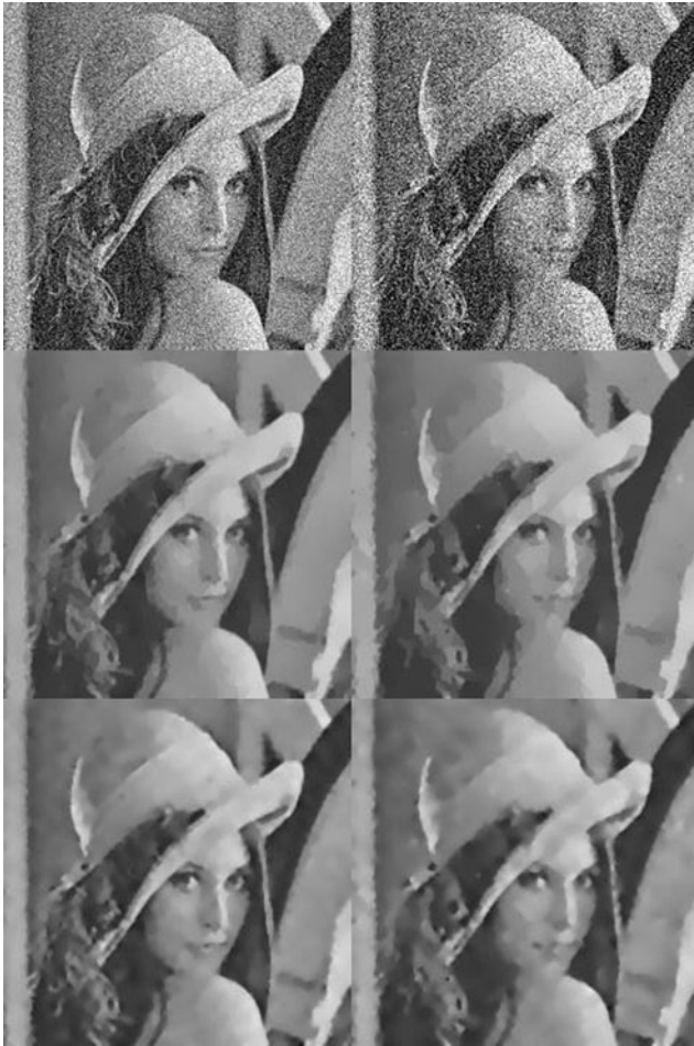
Fig. 9 Denoising results using (2.3) and (4.2) on an image with 20% (left column) and 30% (right column) Gaussian noise. First row: initial noisy images. Second row: results denoising with (2.3). Third row: results denoising with (4.2). The initial clean image can be seen in Fig. 2
