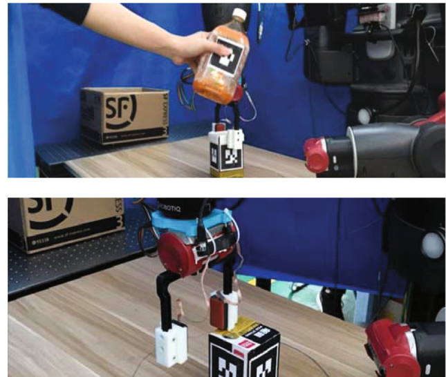
Fig. 1 Anomaly examples when a robot performs a kitting experiment in a shared workspace with a human. Top: an accidental collision between the robot and the human as the human places a new object in the collection area. Bottom: a tool collision as the end-effector prepares to pick an object
