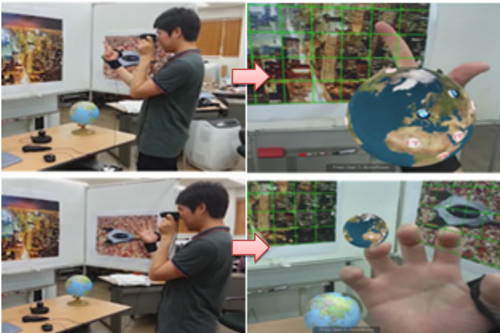
Fig. 1. Bare hand user interaction on video see-through HMD with a RGB-D camera
