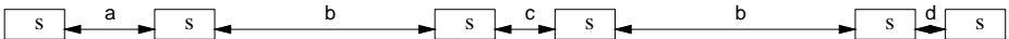
Fig. 4. Parts of a TOPP train. The equally sized probe packets s are sent as pairs with decreasing intra-pair spacing, i.e. d < c < a . The spacing between the pairs are chosen randomly in the range [b - \epsilon, b + \epsilon] where \epsilon is a small number. For each intra-pair spacing, a , c , etc., n pairs are sent.
